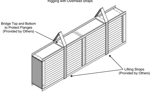
Figure 10 Rigging with Overhead Straps
