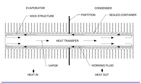
Figure 1 Heat Pipe Section View
