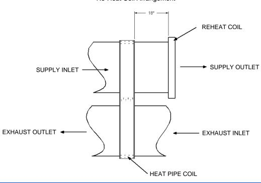
Figure 14 Re-Heat Coil Arrangement
