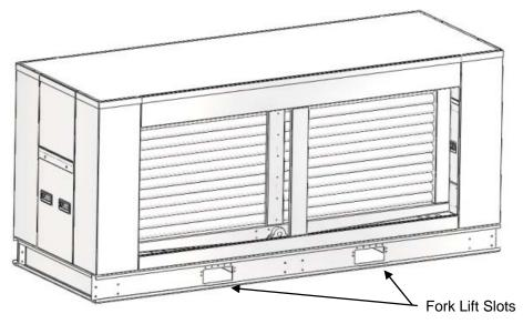
**NOTICE:** Never lift unit by placing forklift in direct contact with the drainpan.
