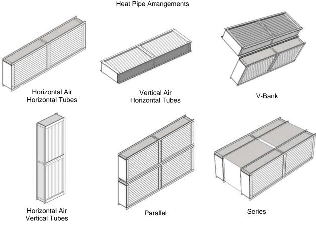
Figure 13 Heat Pipe Arrangements
